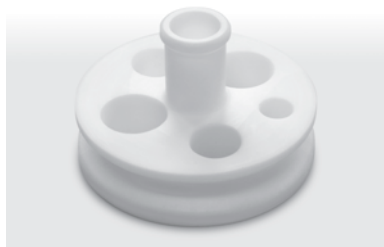
51 161 795 | Teflon® cover for 100 mL reactor, 6 ports 1 x ST10/9, 2 x ST14/23, 2 x ST19/26, center ST14/23
