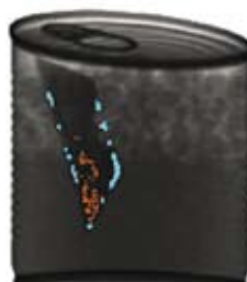
A razor blade is identified in a can of sweetcorn
