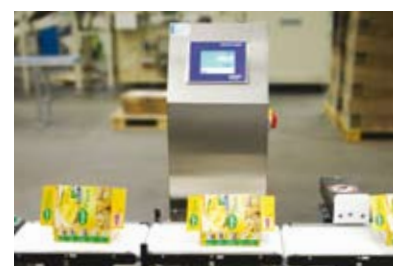
XE3 checkweigher inspects potato products
