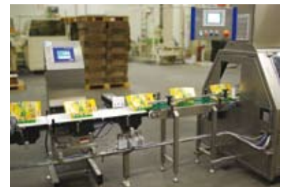
GARVENS XE3 checkweigher upstream of the sealing machine
