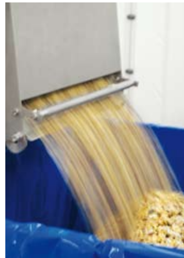
The multi-lane reject mechanism ensures minimal product wastage
