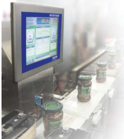
XS3 checkweigher inspects 140 jars per minute
