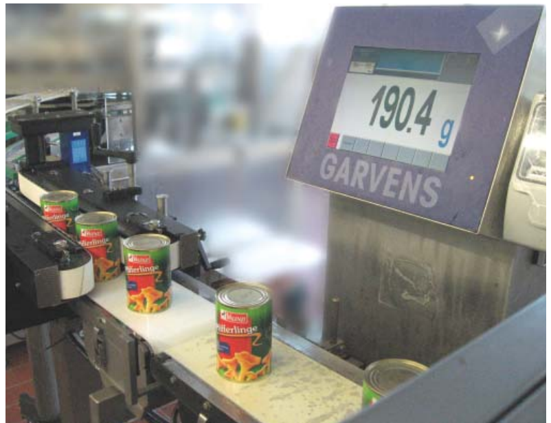
S3 checkweigher inspects tins of mushrooms to ensure the correct product weight is achieved
