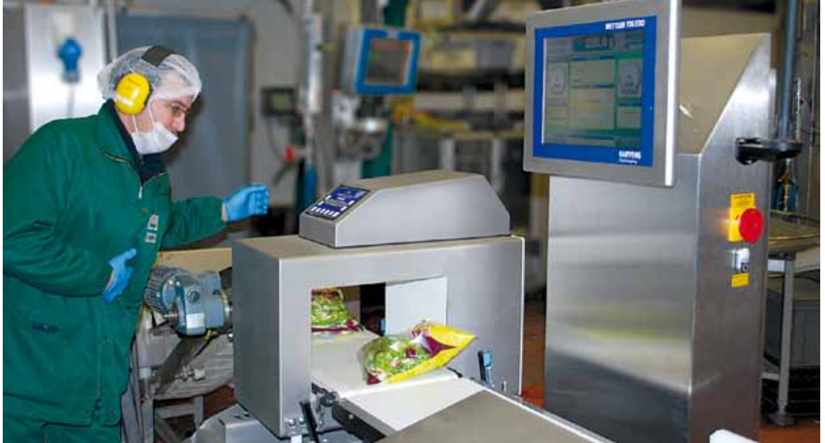
The XS3 CC H CombiChecker inspecting salad in foil pouches
