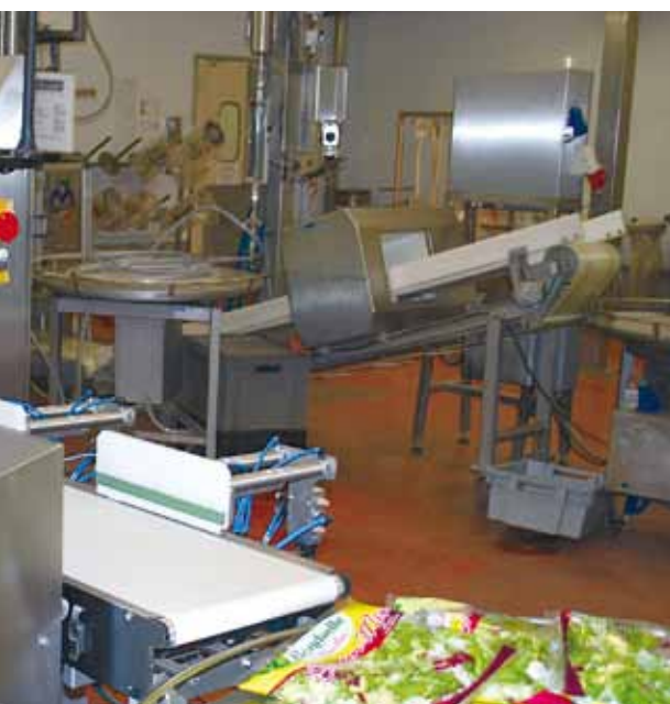
Two pushers with brushes eject defective products from the line – under or overweight products are rejected separately from products containing traces of metal
