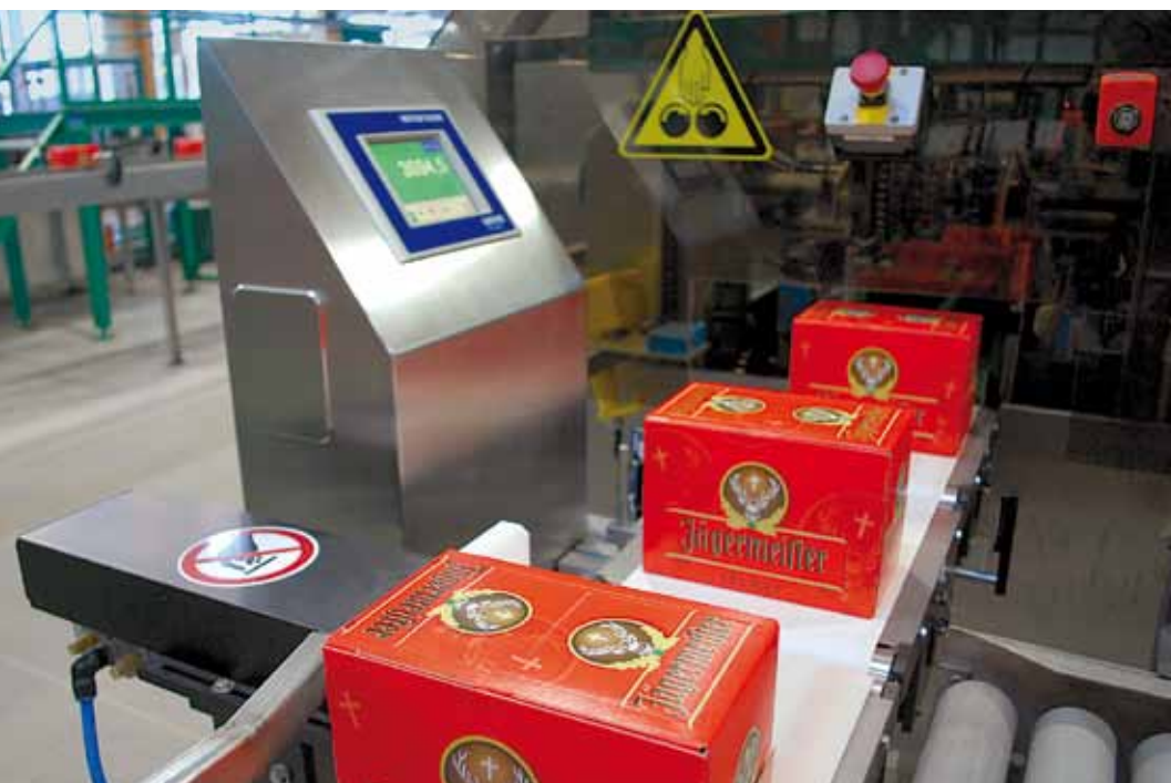
Checkweigher XE3 checking completeness of cartons with bottles
