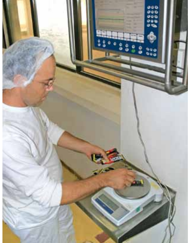
Net content control of Nescafe sticks, Maggi hardtablet bouillon and chokella spread at the FreeWeigh.Net® test places with ID30 PC-terminal
