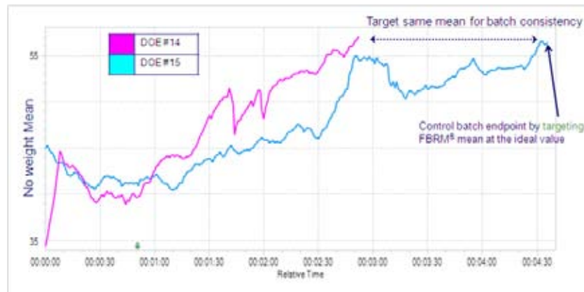
Figure 4 Mean chord length trend for a controlled batch using varying addition rate processing parameters
