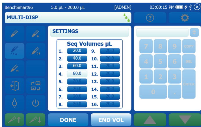
Figure 3-22: Setting the last volume in a sequence
