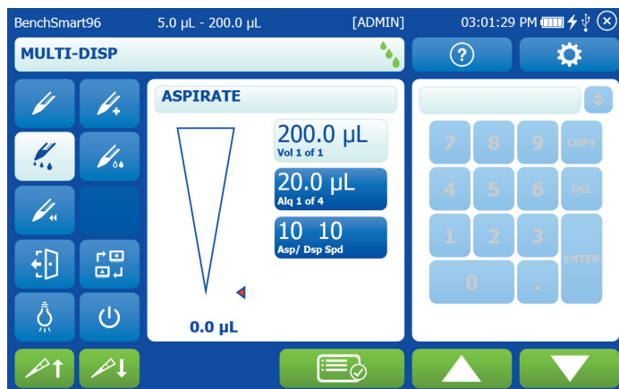
Figure 3-23: Sequential volumes equal to or less than aspiration volume
