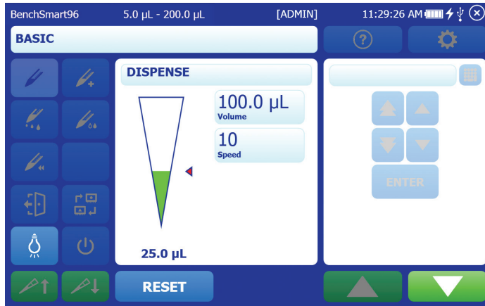
Figure 2-9: Screen depicting dispense volume in tip
