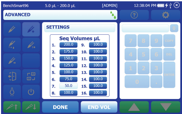
Figure 3-6: Setting the last volume in a sequence
