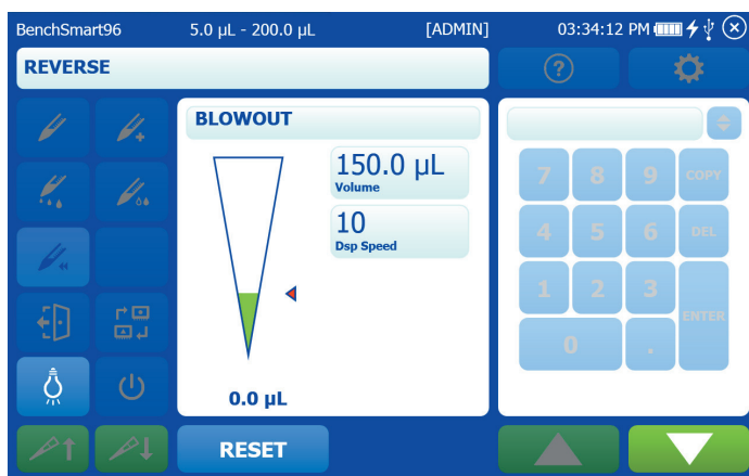
Figure 3-34: Reverse pipetting paused to dispense residual volume
