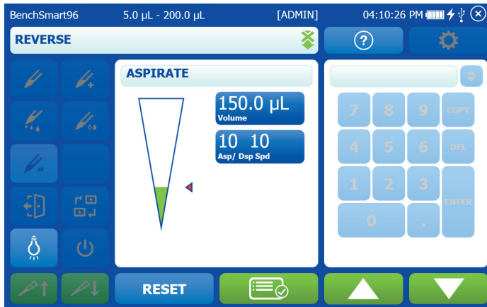
Figure 3-43: Reverse pipetting without "Blowout" option
