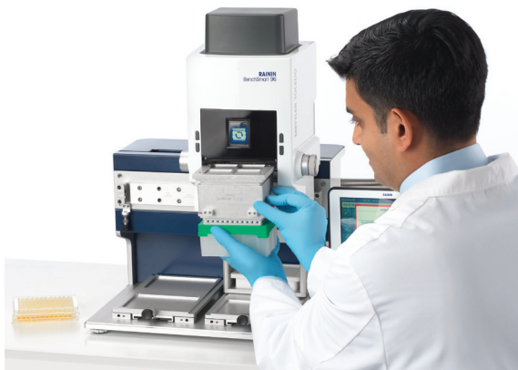
Figure 1-21: Using an empty rack to support the pipette head
