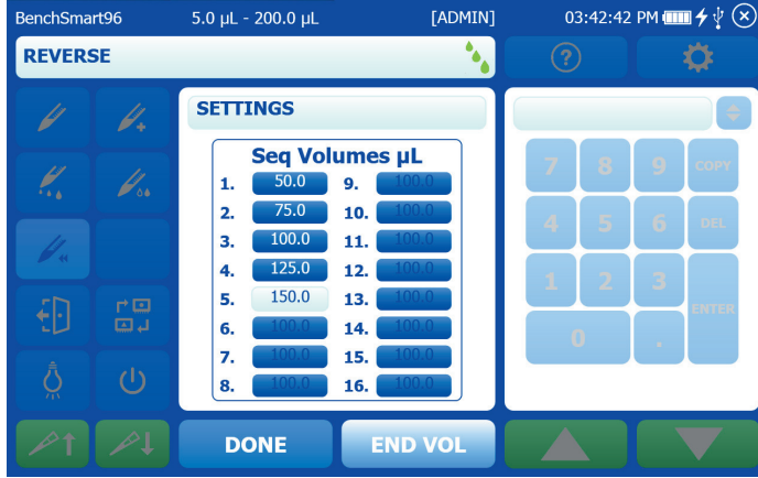
Figure 3-39: Setting the last volume in a sequence
