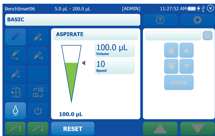
Figure 2-8: Screen depicting aspirated volume in tip
