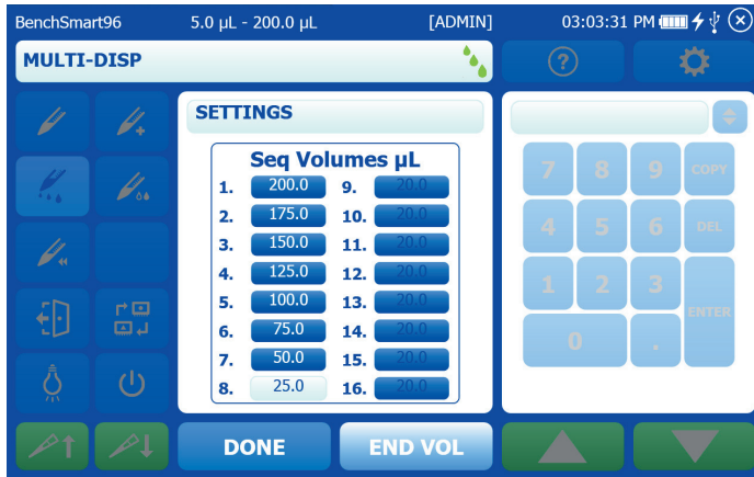
Figure 3-24: Setting the last volume in a sequence
