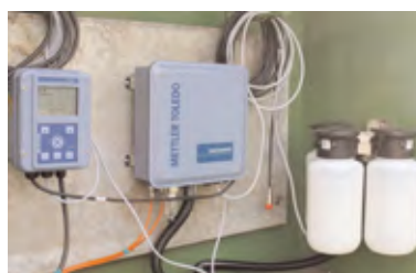
Fig. 1: M 700 transmitter (left) with EC 400 and cleaning solutions. Tubes lead to the housing.
