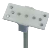
70s Multi-thermocouple DSC sensor for TGA
