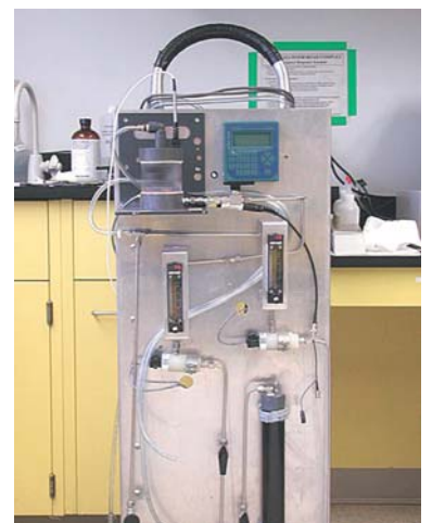
770MAX portable verification system measuring specific and cation conductivity and pH. Dissolved oxygen has since been added to this system.
