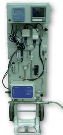
770MAX portable verification system measuring conductivity, pH, dissolved oxygen and TOC with local data acquisition.
