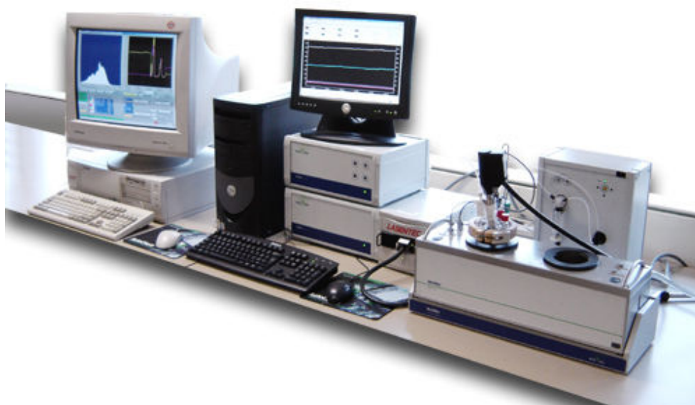
Fig. 1: Reaction setup with one reactor/FBRM probe in an RB02-250 Reactor Box, one Dispenser Box (for antisolvent addition) and the FBRM instrument with one S400 14/206 probe. Two PCs (one PC is possible as well) were linked to allow for data exchange between the two systems and their software packages
