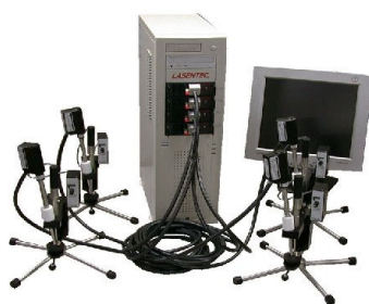
Fig. 3: Lasentec FBRM S 400 Q system with four independent probes.
