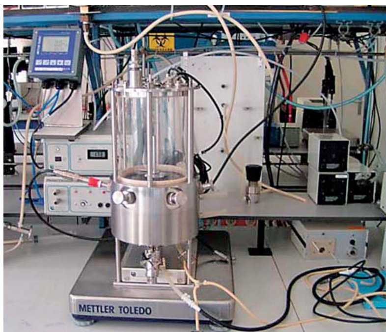
Fig. 1: 4.0 Liter laboratory fermenter with side-mounted CO 2 sensor.
