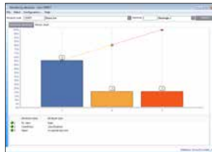
Attributive product defects can also be visualized by FreeWeigh.Net® in the Pareto chart.
