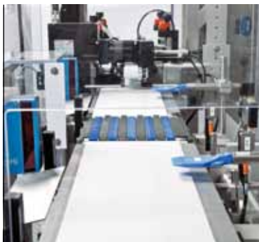
Reliable rejection of "unsatisfactory" products using air jets and rejection counter-check for highest safety
