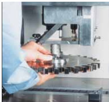
"No tools" starwheel changeout
