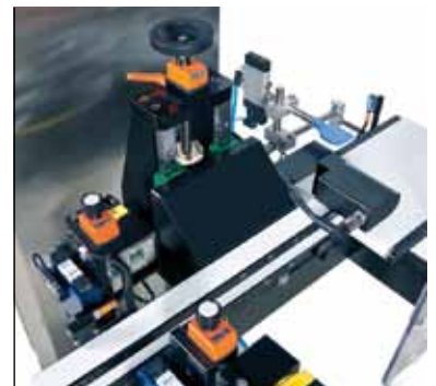
Precision adjustment using numeric indicators for quick and easy adjustment of pass width or height according to package size to speed up product set-up and changeover
