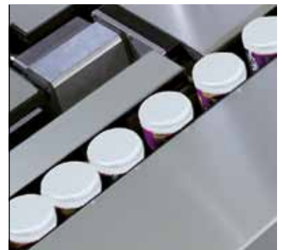
"High performance chain checkweigher" amazing throughput rates – up to 1000 weighings per minute.
